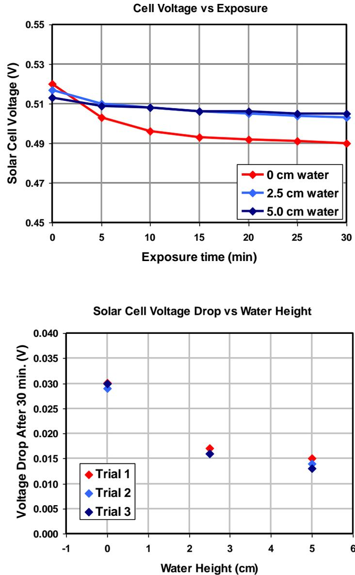
Figure 11. Results of experiment 4 showing the effect of increasing thicknesses of water layers placed above a solar cell on the output voltage of the cell.
