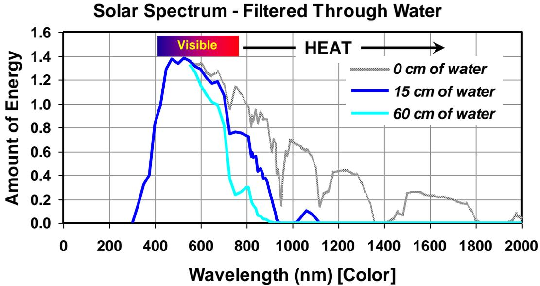
Figure 3. Solar Spectrum-Filtered Through Water.
