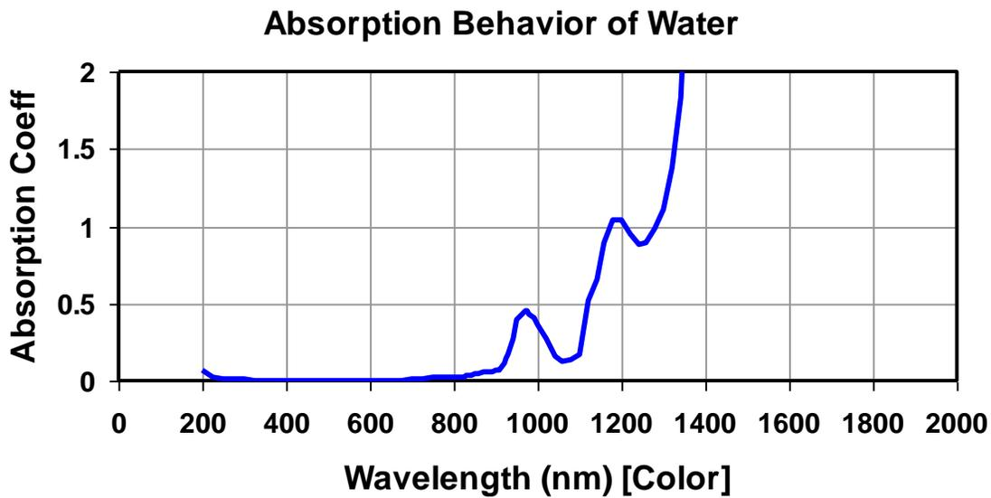
Figure 2. Absorption coefficient of water as a function of wavelength.
