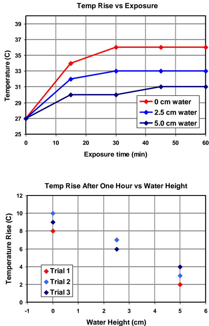
Figure 10. Results of experiment 3 showing the effect of increasing thicknesses of water layers placed outside the window of a house exposed to sunlight on the temperature inside the house.
