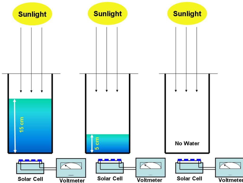
Figure 7. Setup used for Experiment 4.
