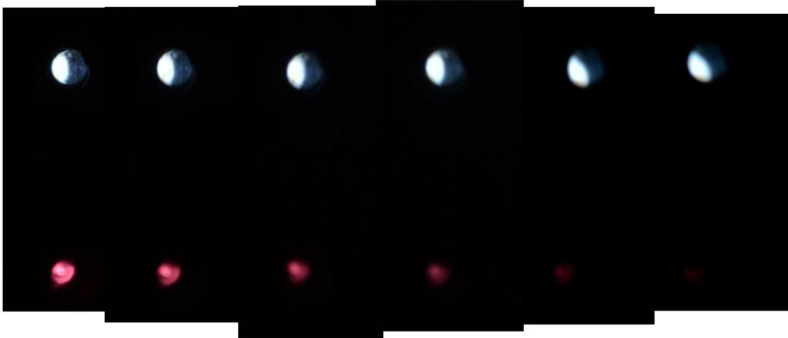
Figure 8. Results of experiment 1 showing IR radiation being absorbed by water while visible light is transmitted with no loss of brightness.
