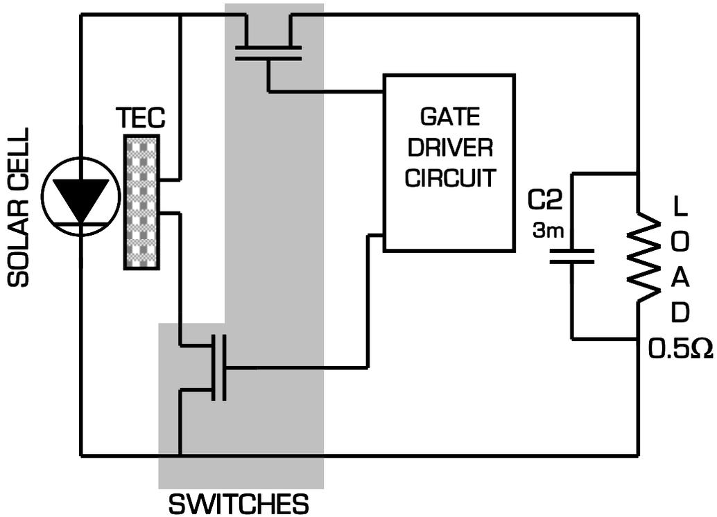
Fig. 12. Diagram showing circuit used to monitor power generated by solar cells.
