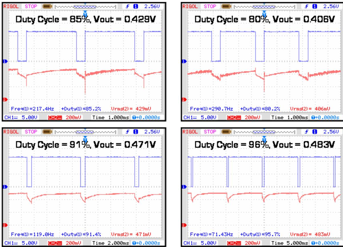
Fig. 21. Voltage waveforms across load (bottom) and gate signal S1 for various duty cycles with self-cooling on.
