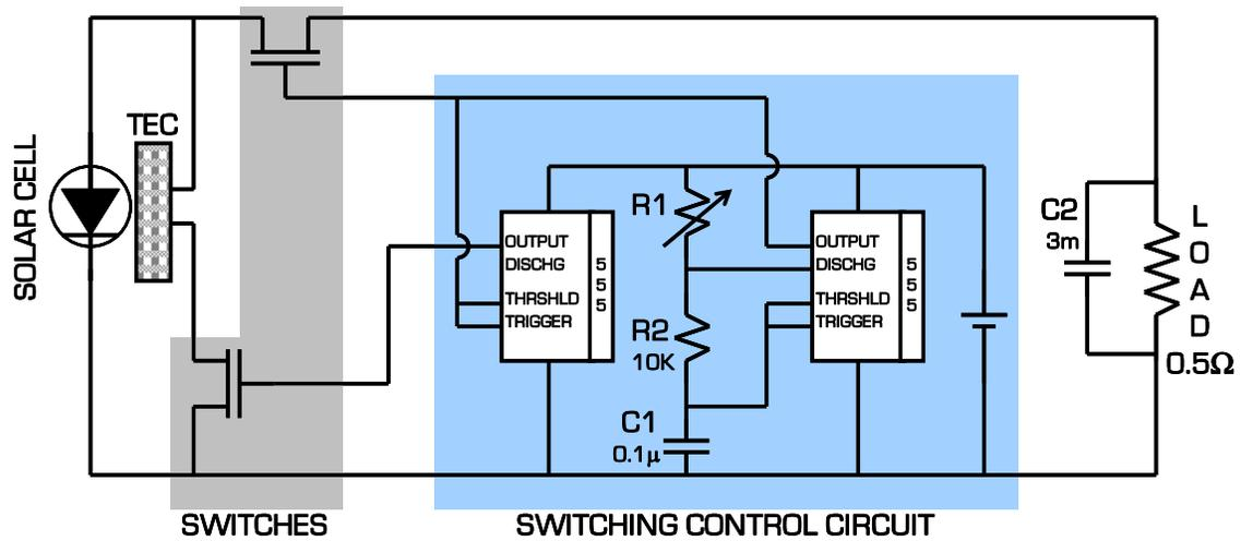
Fig. 13. Circuit schematic showing details of gate driver circuit implementation using 555 timers.
