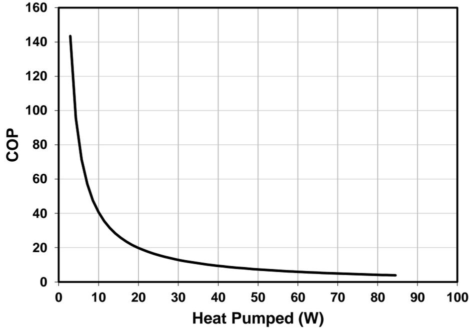
Fig. 8. Theoretically calculated COP versus heat load for a typical TEC module.
