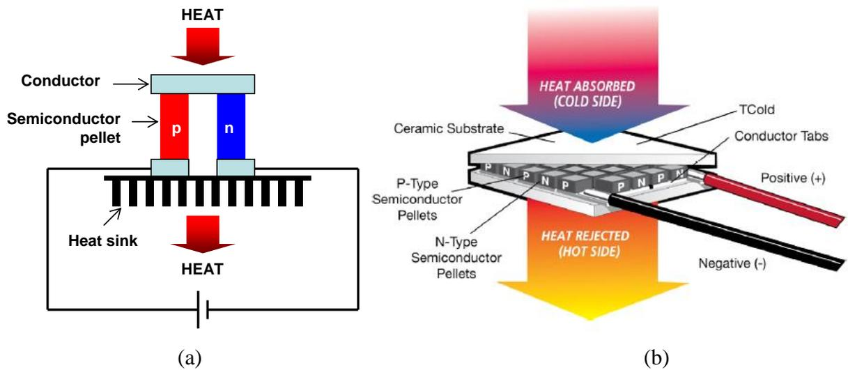
Fig. 4. Simplified diagram of a TEC showing (a) a single junction and (b) an assembled view of a TEC module.
