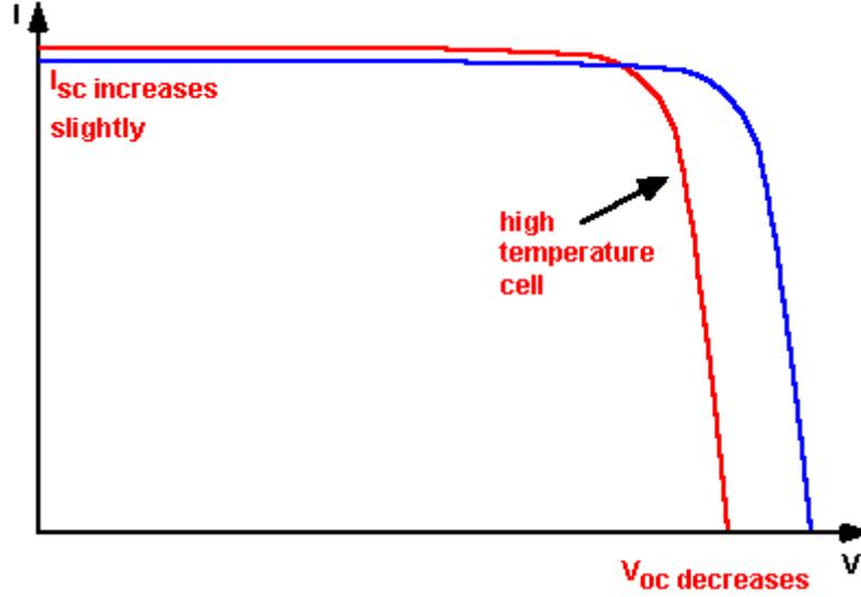
Fig. 3. Typical hot (red) and cold (blue) I-V curves of a PV solar cell.
