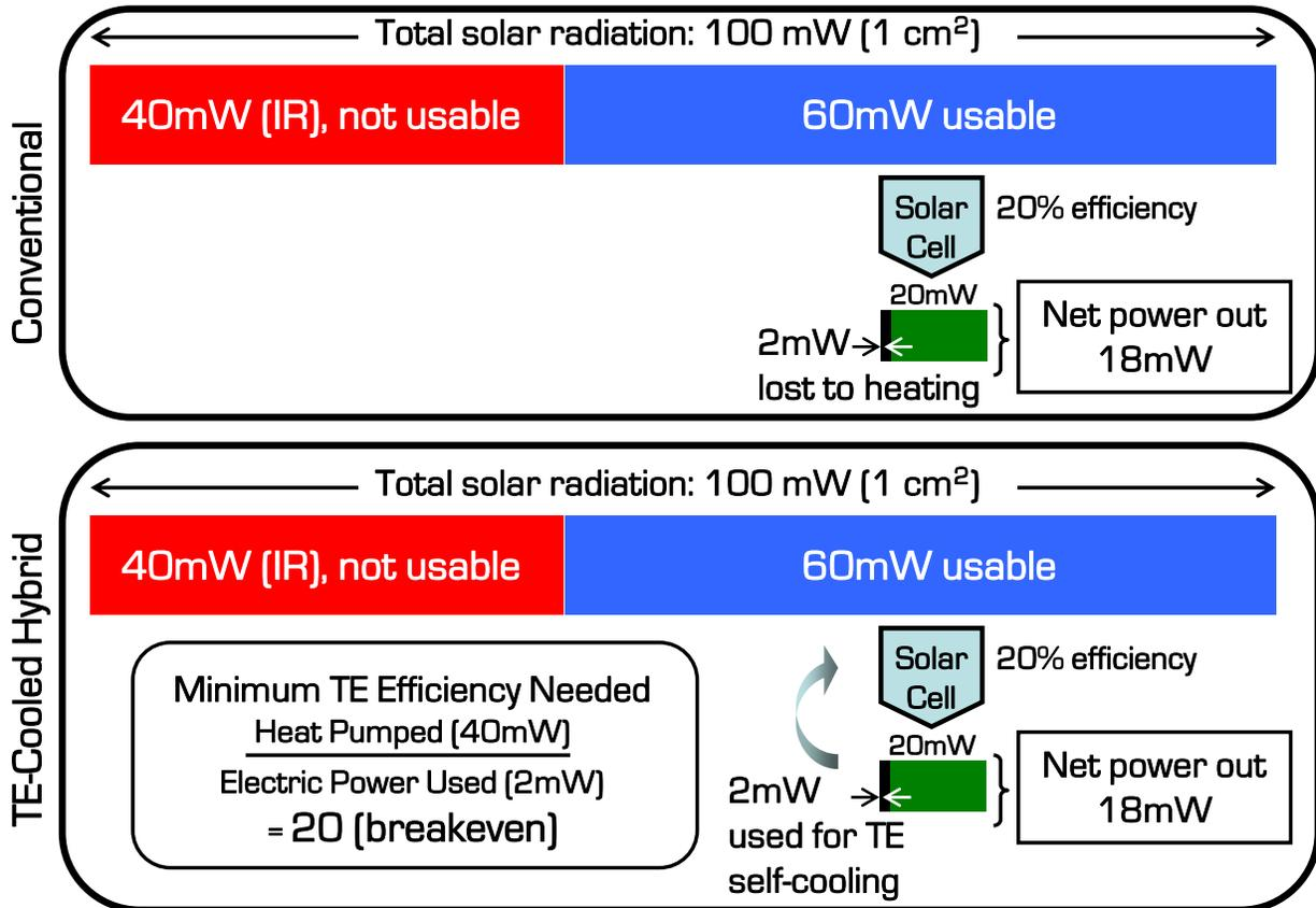
Fig. 7. Pictorial representation of power distributions leading to TEC COP requirement.
