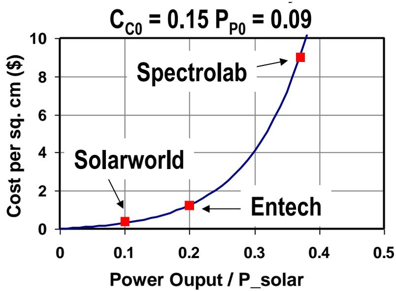
Fig. 24. Model of solar cell cost as a function of cell's output power capacity.
