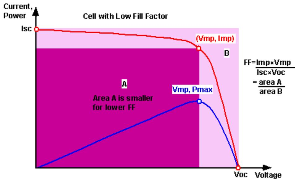
Fig. 2. Typical I-V (red) and P-V (blue) curves of a PV solar cell.
