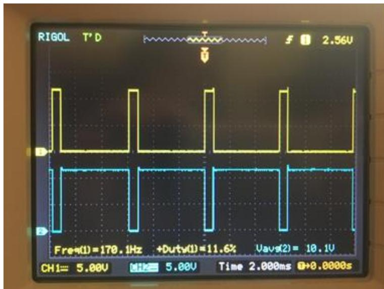
Fig. 18. Oscilloscope waveform of gate drive signals showing correct complementary switching.
