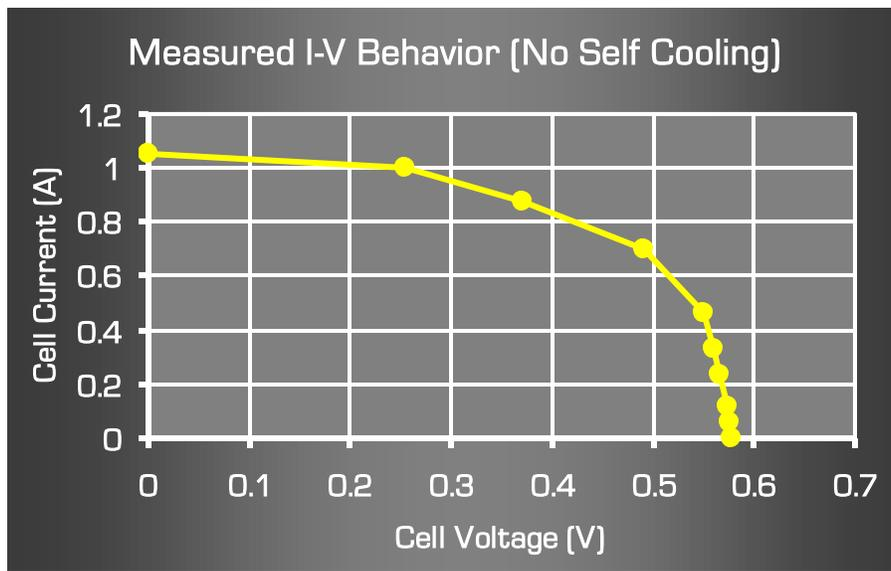
Fig. 16. Measured I-V behavior of a conventional solar cell used to locate the maximum power point.
