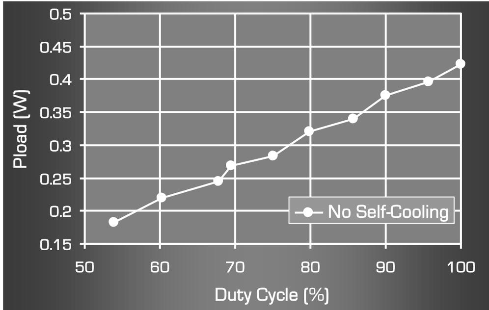
Fig. 20. P Power output versus duty cycle with the TEC module disconnected.
