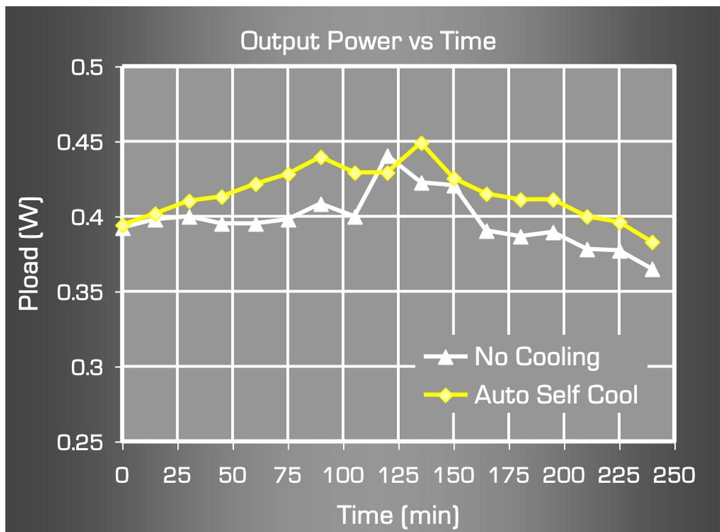
Fig. 23. Variation of power output over time for both conventional and self-cooled solar cell.
