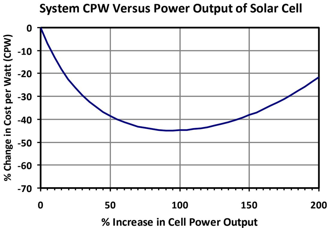
Fig. 25. Analytically modeled variation in the change in CPW as a function increase in cell output power.
