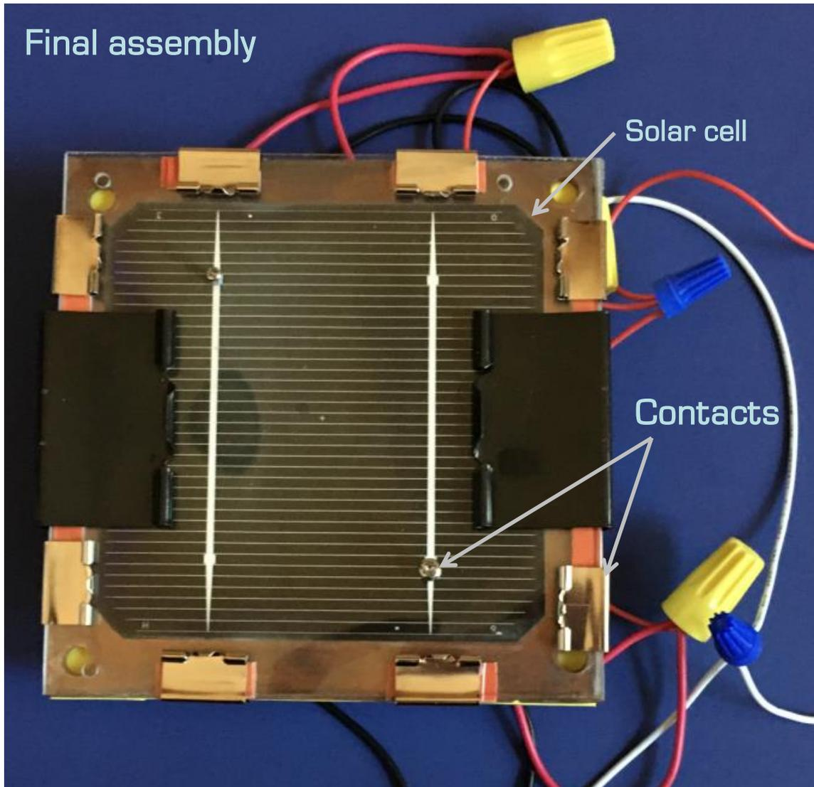
Fig. 10. Photograph of final assembled thermoelectrically cooled solar cell.
