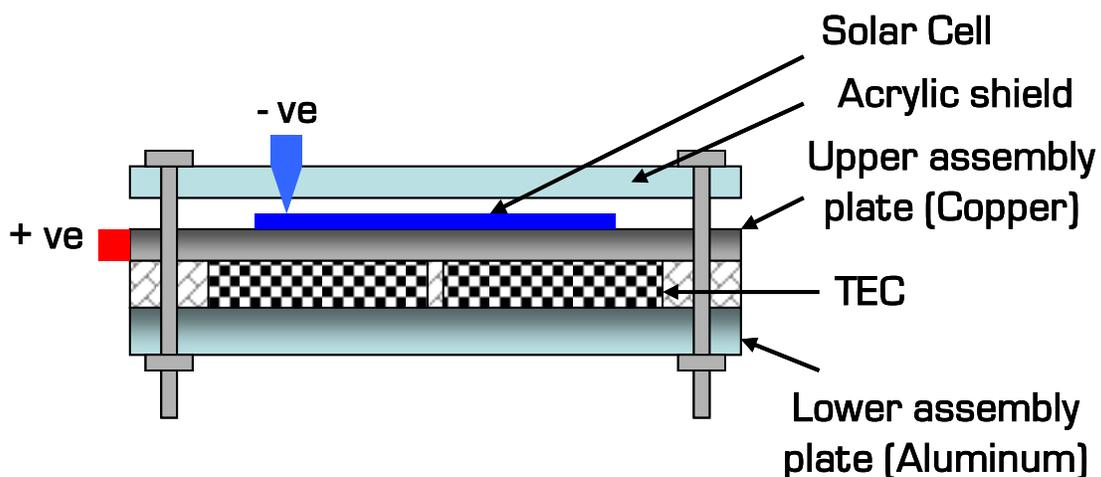
Fig. 9. Diagram showing details of how the self-cooled solar cell is assembled.
