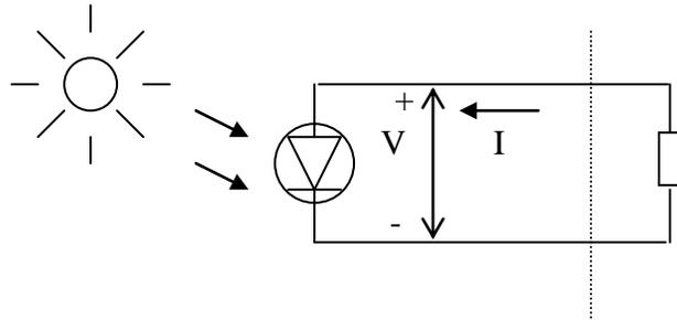
Fig. 1 Simple equivalent circuit of a photovoltaic solar cell.
