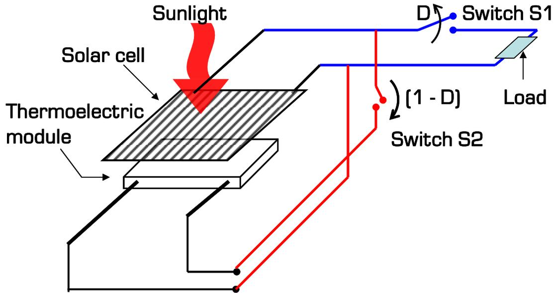
Fig. 11. Conceptual schematic of switching circuit used to divert a portion of the solar cell power output to the thermoelectric cooling module.
