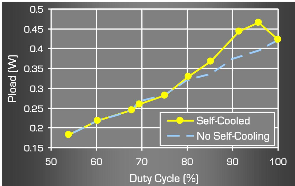
Fig. 22. Power output versus duty cycle in a self-cooled solar cell. Power output peaks at about 96% duty cycle. At this duty cycle the power output is 10.25% higher than without cooling.
