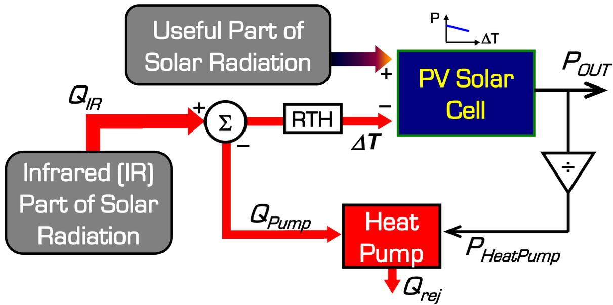
Fig. 5. Conceptual view of self-cooling approach used in this project.
