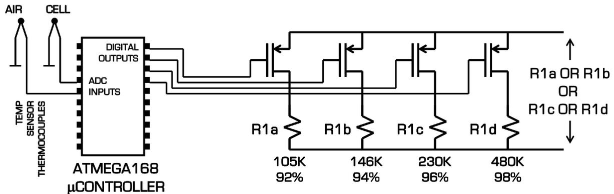
Fig. 14. Schematic drawing of the digital duty cycle control circuit.
