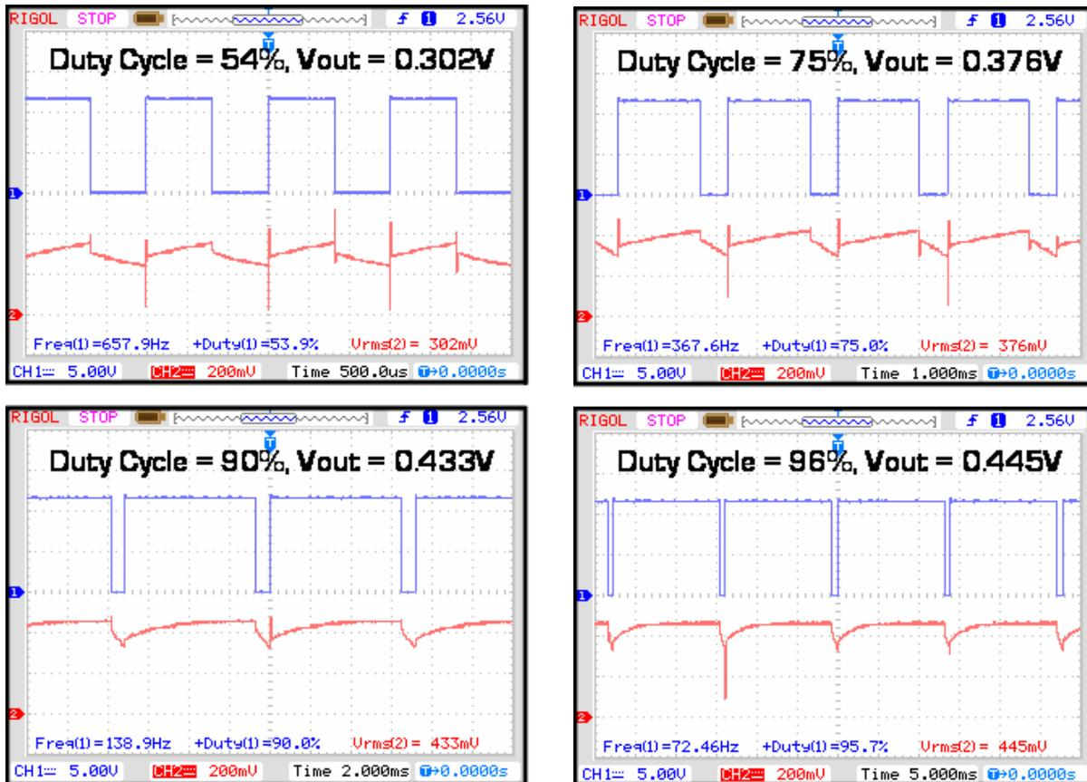
Fig. 19. Voltage waveforms across load (bottom) and gate signal S1 for various duty cycles.
